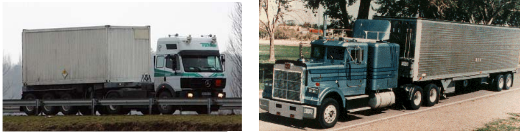
Comparison of French (left) and United States road transport vehicles - the French vehicle is a commercial tractor unit with an unarmoured ISO container on the trailer - the US safe secure transport (SST) is a fully armoured custom-built vehicle with anti-access and removal equipment and devices built-in - the US vehicle is limited to 3 FS47 flasks whereas the French vehicle carries 9/10 FS47 flasks. The US SST shown may now have been replaced with a similar but upgraded SGT vehicle.
